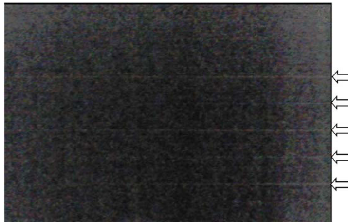
Figure 1. Row Noise at Low Light Condition
