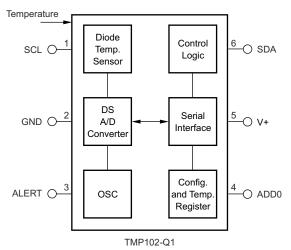
Figure 1-1. Functional Block Diagram
