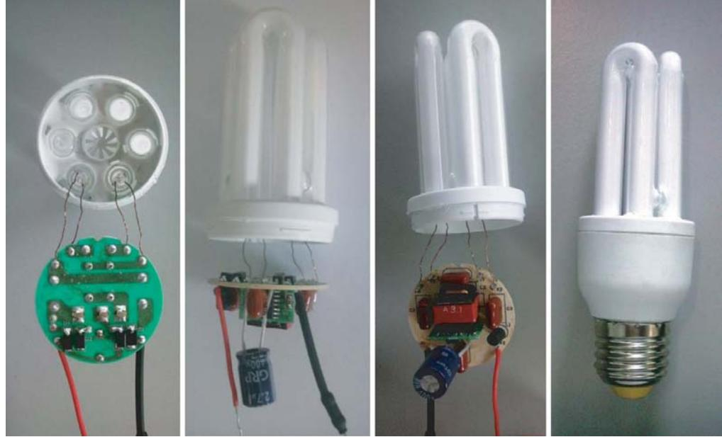
**Fig 2.** Photos of a 12 W CFL with the UBA2211
