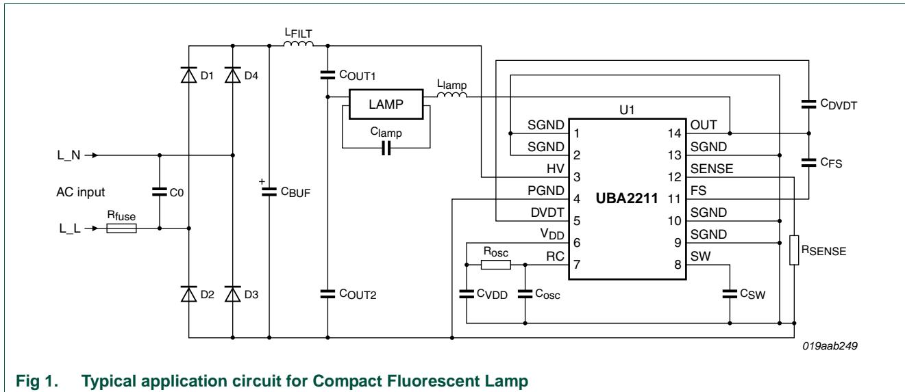
**Fig 1.** Typical application circuit for Compact Fluorescent Lamp
