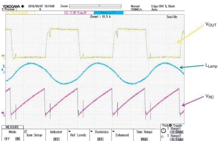
Fig 11. Capacitive mode protection in RMS state
