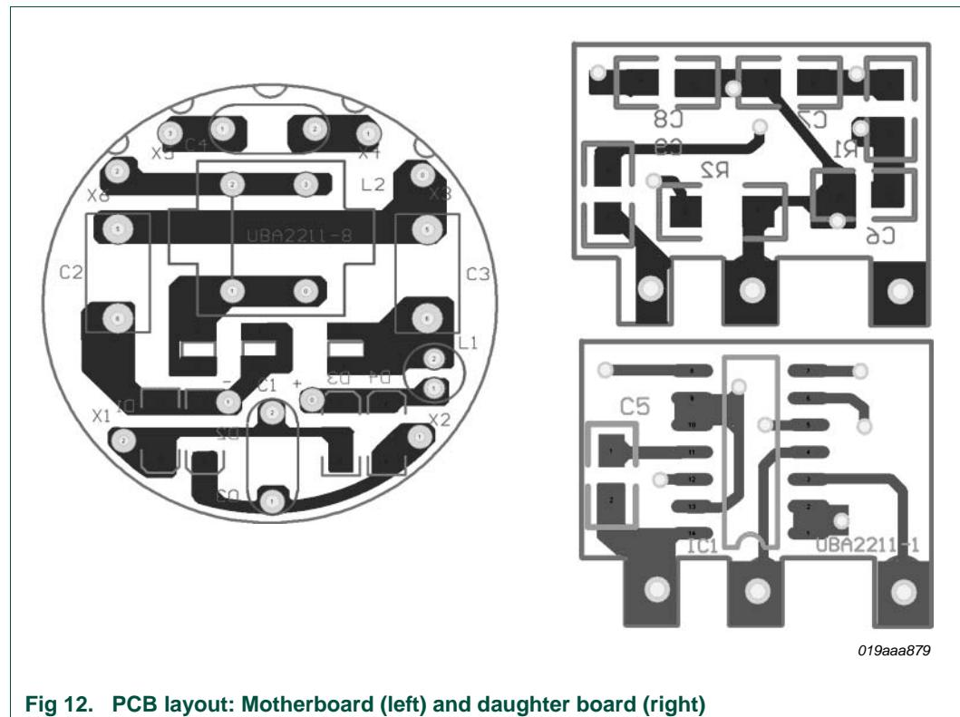
Fig 12. PCB layout: Motherboard (left) and daughter board (right)
