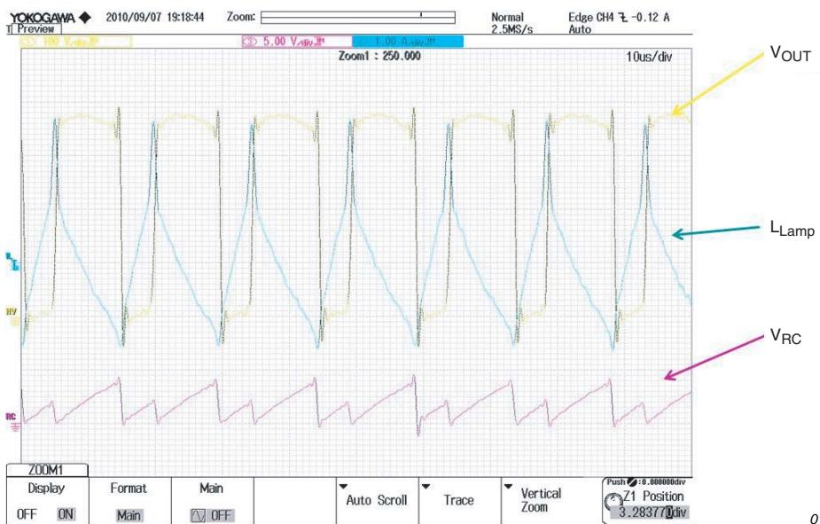
Fig 10. Correctly functioning IC with saturated inductor at ignition
